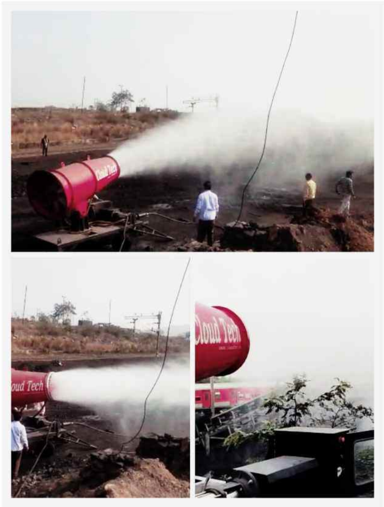
Trolley mounted fog cannon at railway siding
